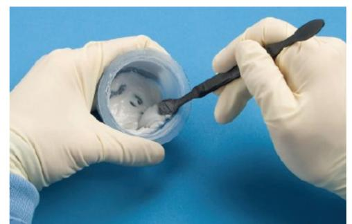
Vigorously mix the powder and solution in a circular motion for 45 seconds, ensuring that all of the solution has been distributed throughout the powder.
