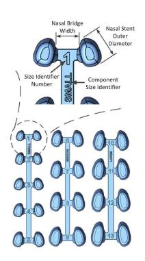
Each sizer component has identifier numbers which correlate to the nostril retainer size they represent. The sizers are designed to represent the nasal stents (when trimmed) and bridge width (distance between right and left nasal stents) for all retainer designs.
